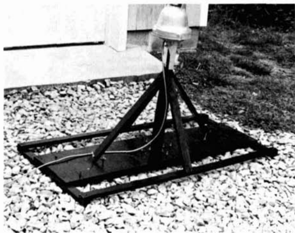
fig. 4. Assembly, supported by four braces, mounted on 2x4-foot (60x120cm) plywood frame for fastening to flat area. TR-44 rotor can be mounted on regular tower. Length of mast from TR-44 to U-100 should not exceed 5 to 6 feet (1.5-2 meters).
